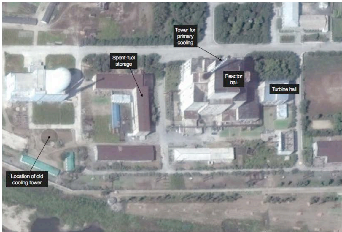
Fig. 3. Physical layout of the 5MWe reactor at Yongbyon (image from Google Earth, 9/24/2014; CR 2015 DigitalGlobe).
