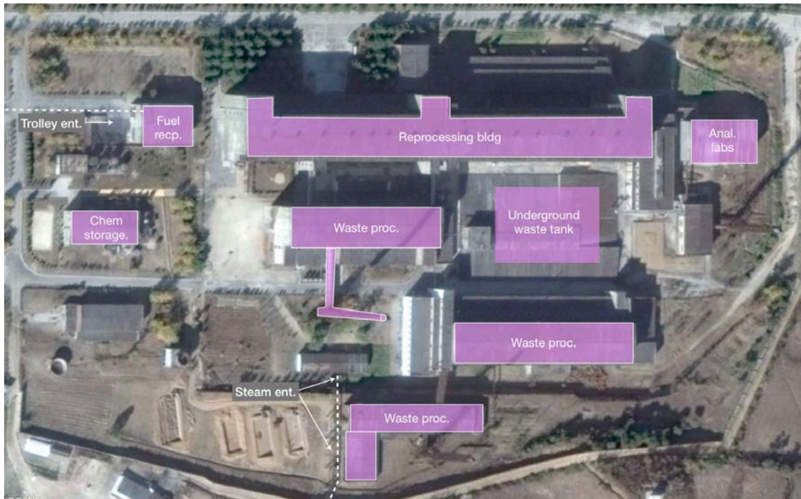
Fig. 12. Layout of the radiochemical complex (image from Google Earth, 10/27/2014, CR 2015 DigitalGlobe).
