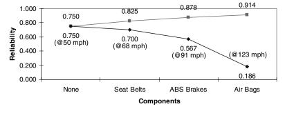
Fig. 6. Overcompensation and reduced component reliability.
