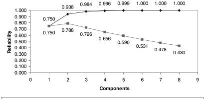
Independent Redundant Components Placed in Parallel (0.75 base component reliability)
