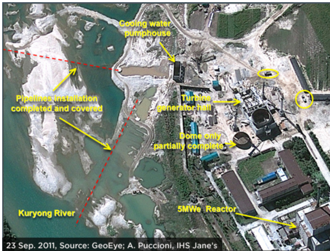
Annotated diagram of the new reactor site, shown in a photo indicating significant progress in construction.
